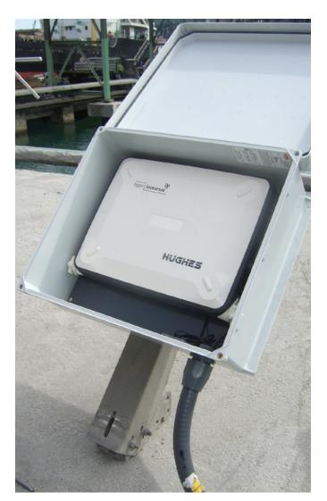
The Hughes 9201 M2M Satellite Terminal is your gateway to global machine-to-machine communications. The 9201 M2M enables you to simultaneously send and receive IP packet data via Ethernet over the Inmarsat BGAN satellite network.
